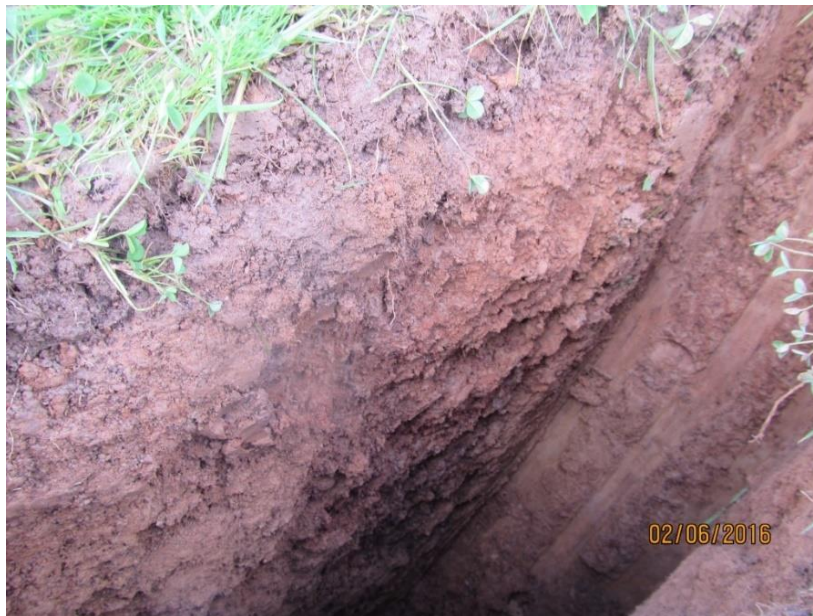
Figure 1. Typical Red Brown Earth in the Riverine Plain with medium or heavy clay subsoil, dispersive subsoil conditions and low or slow rates of permeability.
